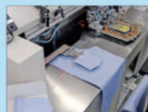
1. 摆放口袋裁片(免烫) Laying the cut piece of pocket(iron-free)
