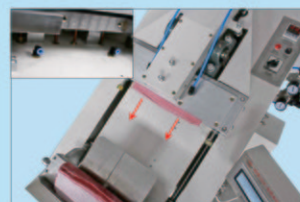
吹风自动收料 Air blowing facilitates automatic cuff collection
