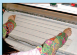
可同時對襯衫前筒及口袋 進行粘壓 Shirt front placket and pocket can be fused and pressed simultaneously
